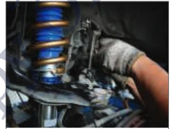
▲ Figure 14 One type of suspension unit used in motor vehicles. The blue cylinder inside the spring is the damper (shock absorber) and usually consists of a piston filled with oil.
