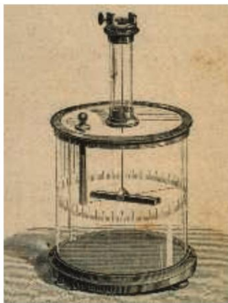
▲ Figure 6 The apparatus used by Charles-Augustin de Coulomb to show that the force between two charged objects obeys an inverse square law.
