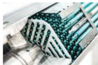
▲ Figure 8 These bundles of fuel rods for a nuclear reactor are about 0.5 m long and 0.1 m in diameter. Each bundle generates about 4 Tj of energy during the time it is in the reactor.
