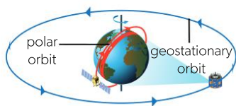
▲ Figure 60 Satellites in orbit. The polar orbit takes about 90 minutes. A geostationary satellite orbits once in 24 hours and so appears to sit at one point above the equator.
