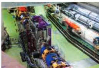
▲ Figure 18 Particle accelerators such as this picture of the ALBA synchrotron in Spain cause charged particles to move in circles. They must be accelerated and therefore emit electromagnetic radiation called synchrotron radiation.
