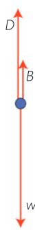
◀ Figure 34 A sphere dropping through a viscous liquid has its weight W , a buoyancy force B , and a drag force D acting on it.
