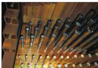
► Figure 11 Organ pipes of various sizes. The circular pipes are open at both ends, whereas the square pipes are closed at one end. The metal collars on the round pipes can be moved to enable a fine adjustment in the tuning. The square pipes have a plunger for this.
