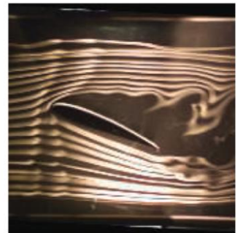
▲ Figure 33 A model of an aircraft wing in a wind tunnel. The wing is at an angle such that the air flow around it becomes turbulent.
