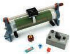
▲ Figure 24 A variable resistor; also called a rheostat. It has three terminals: one at each end of the resistance coil and one connected to a slider that touches the resistance coil.
