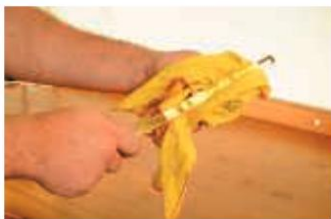
▲ Figure 4 Transferring charge by friction. The Perspex rod and the cloth are initially uncharged. After rubbing the cloth on the rod, the Perspex is positively charged and the cloth is negative.
