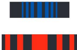
▲ Figure 20 Two diffraction patterns produced by the same slit but with different wavelengths. Blue light has a shorter wavelength than red and the diffraction pattern formed with blue light spreads out from the centre less than the red pattern.
